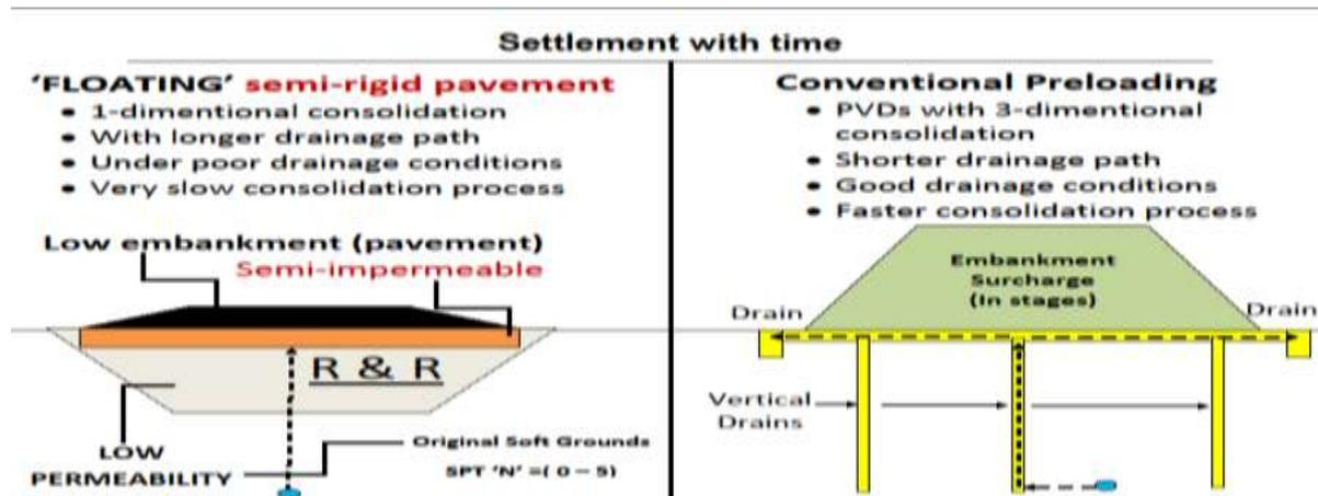
Fig 1: 'Floating' platform to reduce total settlement and minimize different settlement.
