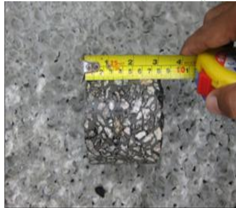
(b) Thickness Measurement of the Sample (75mm thick)
