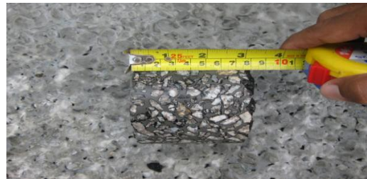
Fig. 6b Coring samples (75mm thick)
