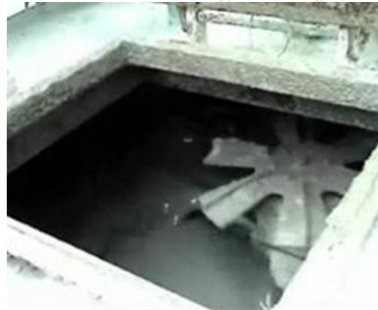
Mixing cement mortar with water at W/P ratio of 0.30~0.31
