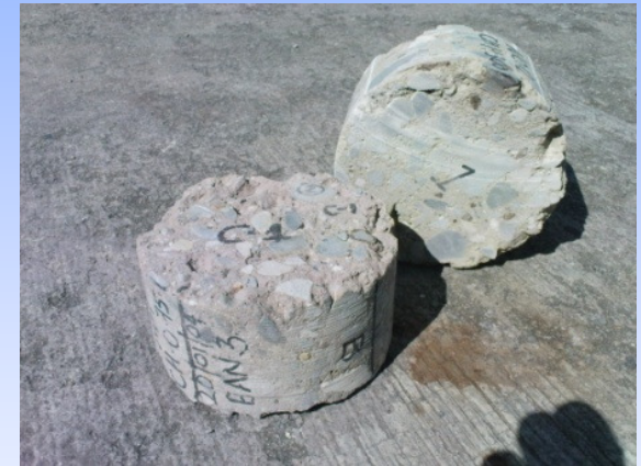
c) Cored Samples stabilized Recycled Materials
