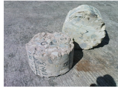
c) Cored Samples stabilized Recycled Materials
