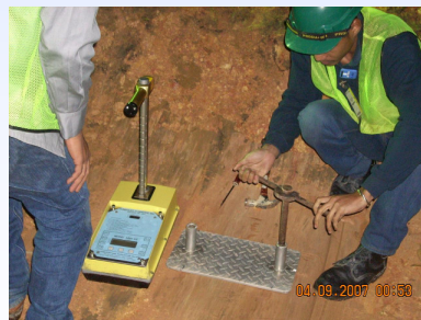
Photo 16. Nuclear Density Test
