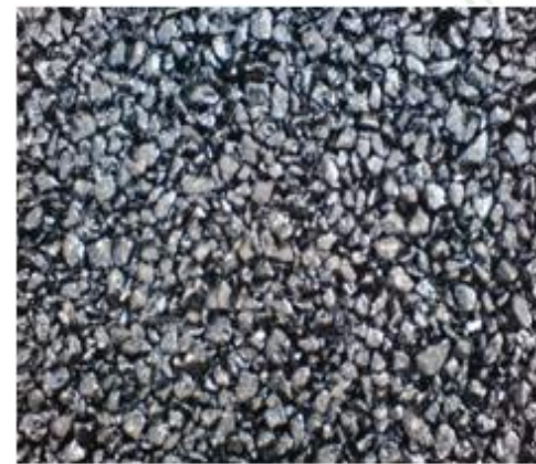
(f) Compacted PAC Surface (Air Void 25-30%)
