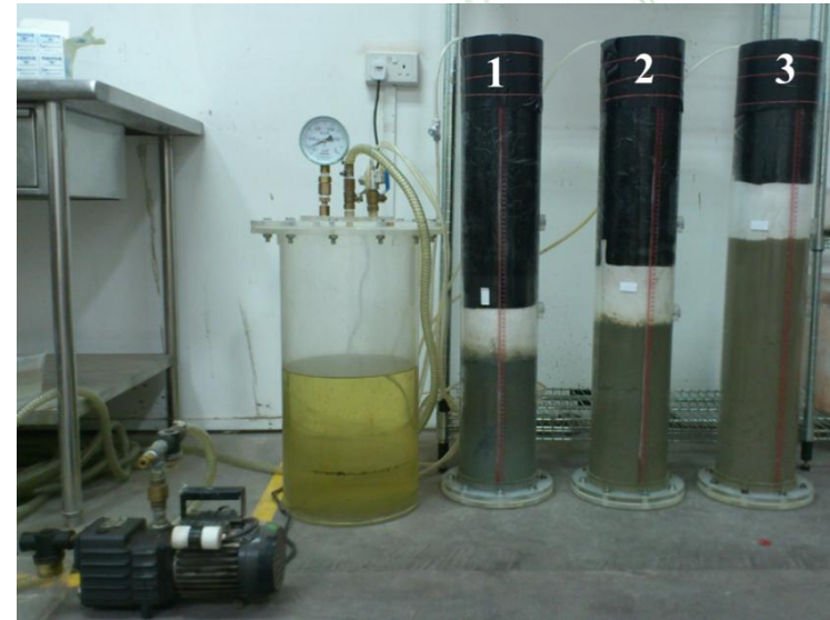
FIG. 1a. 3-D NFS Consolidation Test by VP (1: Sand; 2: Geotextile; 3: Vertical drain; 4: Clay samples; 5: Pressure control valve; 6: Vacuum control valve; 7: Pressure Meter; 8: Tubes; 9: Ruler.)
